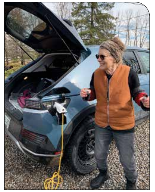
During the derecho of 2022, Sue Brandum plugged her Hyundai Ioniq 5 into her neighbour Laura Plummer’s sump pump to keep Laura’s basement from flooding while her power was out. The feature is called Vehicle to Load, but not all EVs have it. This photo of Laura was taken at the time.
